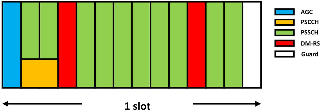
**Fig. 3.** A slot format without PSFCH. Normal cyclic prefix is assumed.
