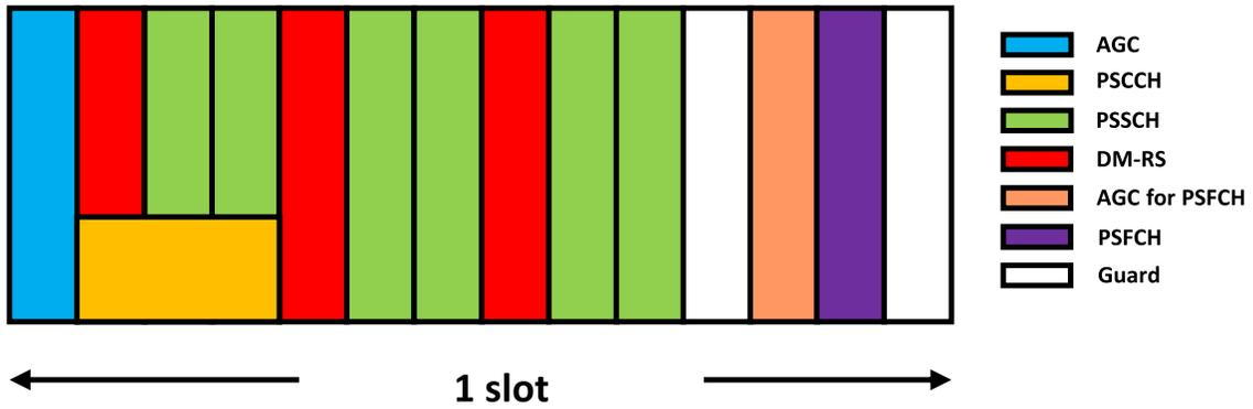
**Fig. 4.** A slot format with PSFCH. Normal cyclic prefix is assumed.
