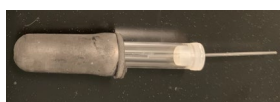
Figure 1. Photograph of a capillary micropipette and squeeze bulb pycnometer assembly used for dispensing fluid.
