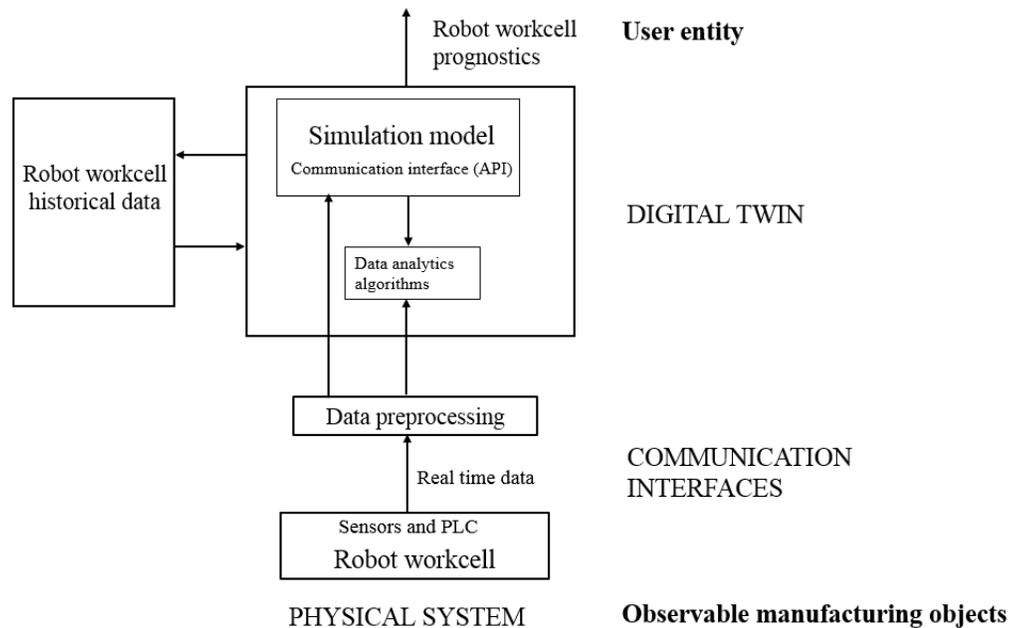
Figure 6: Illustration of relationships between different components of the digital twin.
