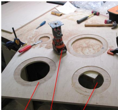
counterbore router clearance hole
