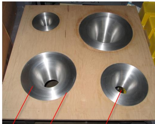
nozzle base silicone sealant nozzle throat
