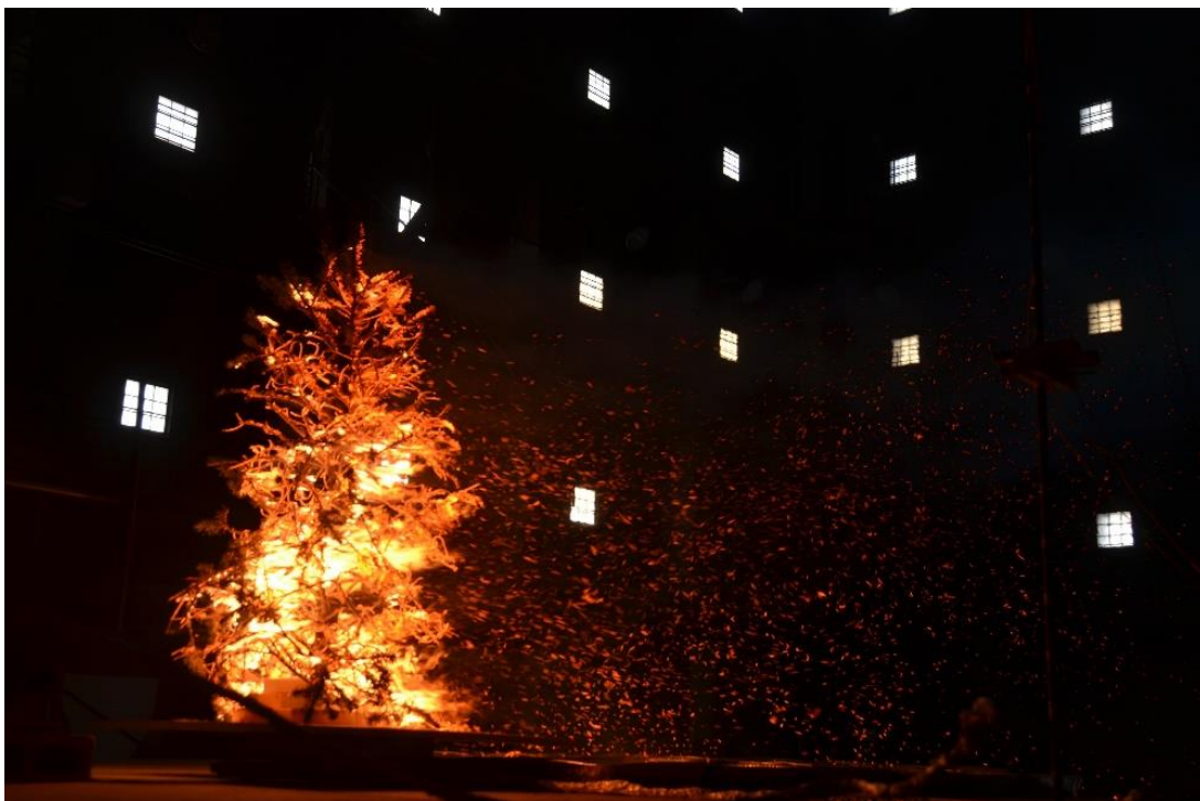
Figure 2 The top image shows the combustion process just after burner application and the bottom image shows the extensive firebrand generation processes. In this experiment, was applied wind speed was 3 m/s. The burner was applied for 10 s.
