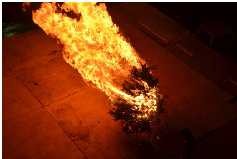
Figure 4 The combustion process of 1.5 m Noble-fir tree after ignition from firebrand showers. In this experiment, a 3 m/s wind was applied, and firebrand showers were selected to be commensurate to burning structures.
