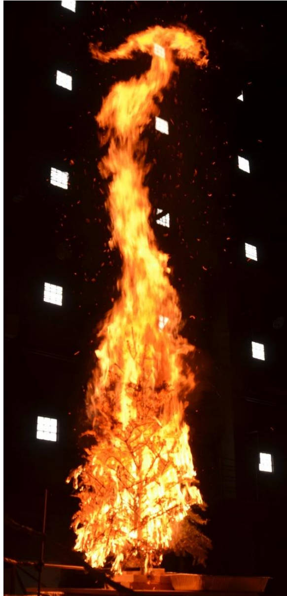
Figure 3 The combustion process just after burner application for a 1.5 m Noble-fir tree. In this experiment, no wind was applied. The differences are apparent in comparison to experiments under an applied wind field (see Figure 2 ). The burner was applied for 10 s.
