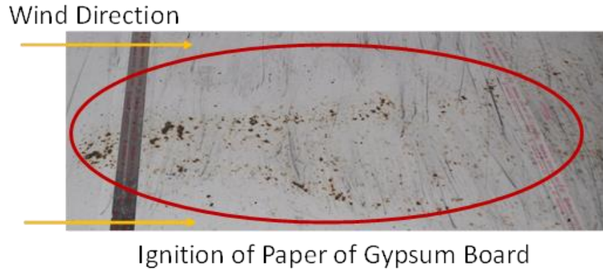
Figure 6 Accumulated firebrands swept off after the completion of the experiments. Ignition points of the gypsum board paper are observed. Douglas-fir wood pieces were used to simulate vegetative firebrands, wind speed of 6 m/s, and the obstacle was 1.32 m (H) by 2.44 (W) [5].
