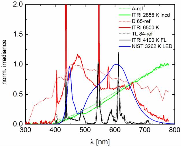
Fig 2. The normalized spectra of the three light sources used in ITRI's indoor lighting simulator and the white LED used in NIST's simulator. The reference spectra are shown in dashed lines for comparison.
