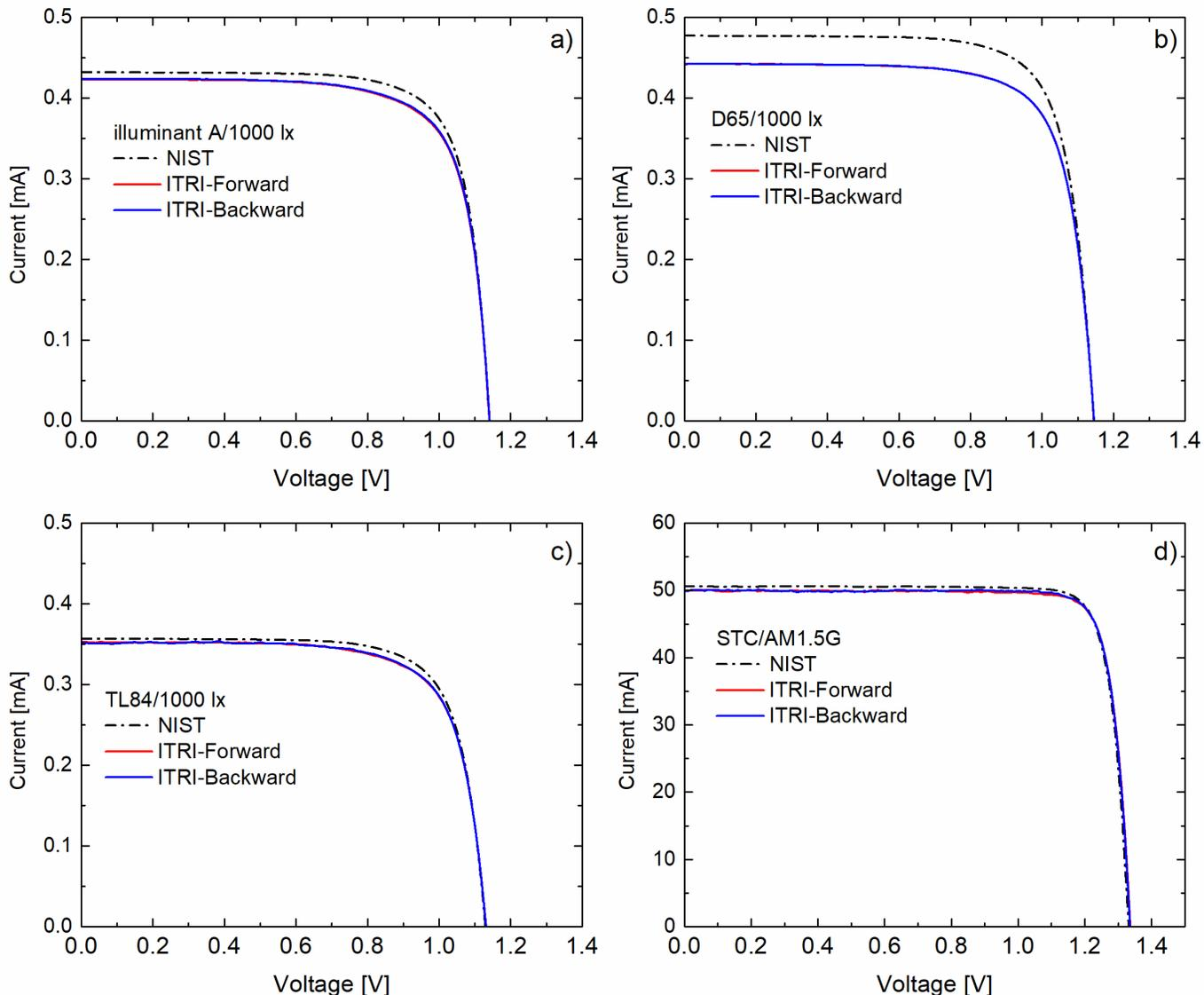
Fig 6. The summary of I-V curve measurements reported by each laboratory under 4 different reporting conditions.
