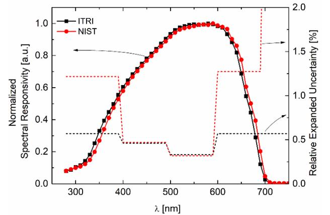
Fig 5. The normalized spectral responsivity curve of the NIST 1005 test cell as measured by NIST and ITRI. Relative expanded uncertainties are also reported.
