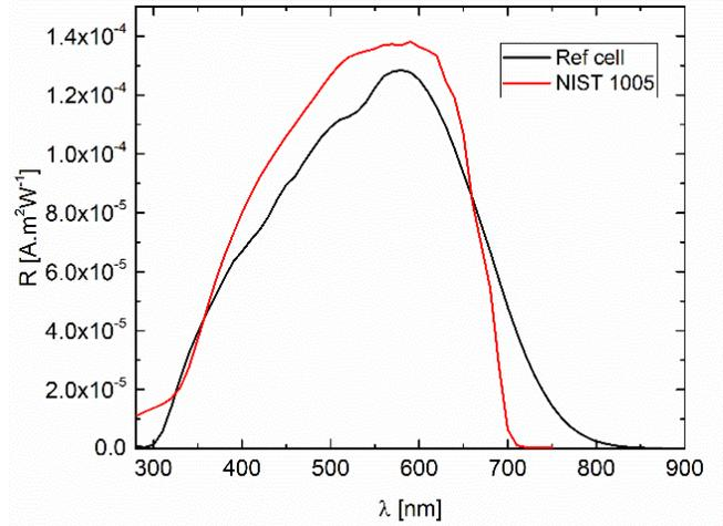
Fig 3. The irradiance-mode spectral responsivity functions of the KG-5 filtered Si reference cell and the GaInP (NIST 1005) test solar cells.
