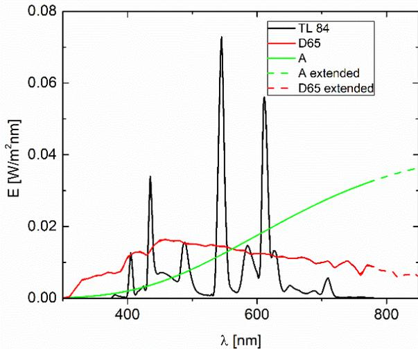
Fig 1. The reference spectra of the three standard light sources used for this interlab comparison. The irradiance values are calculated such that the illuminance produced by each spectrum is exactly 1000 lx.
