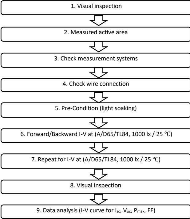
Fig 4. Testing flow-chart and protocol followed by ITRI
