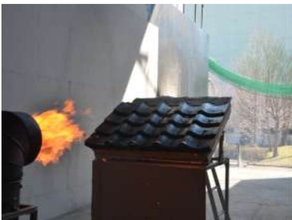
Figure 2 Image of a typical experiment. Applied wind speed of 6 m/s. 2 kg of water was sprayed onto the tiles just prior to the start of the experiments.
