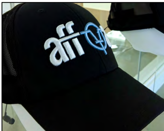
IR Active LOOKs cap that collects a wearer's physiological data through an Apple watch, and optically transmits that information to a third party in real-time. Credit: AFFOA.
