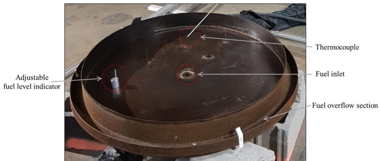
Figure 2. The round, 1 m diameter, water-cooled, steel burner with fuel level indicator and fuel overflow.
