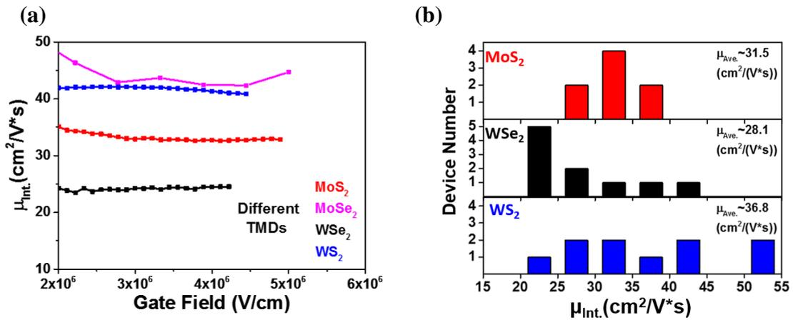
**Figure 4.** (a) Comparison of  $\mu_{int}$  vs. gate field for representative SB FETs from four different TMDs. (b) Histogram of mobilities extracted from 4-terminal measurements for MoS<sub>2</sub>, WSe<sub>2</sub>, and WS<sub>2</sub> devices.
