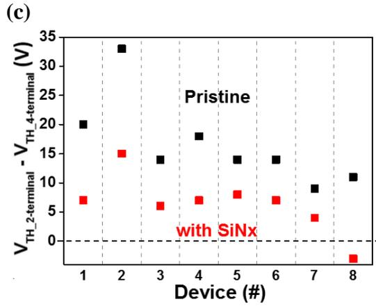
**Figure 5.** (a) Comparison of  $R_C$  as a function of overdrive voltage for a pristine device and the same device after n-doping. (b) Comparison of 2- and 4-terminal linear  $I_{DS}$ - $V_{BG}$  curves after SiNx n-doping treatment. (c) The disparity between 2- and 4-terminal  $V_{TH}$  for eight different devices before and after SiNx doping.
