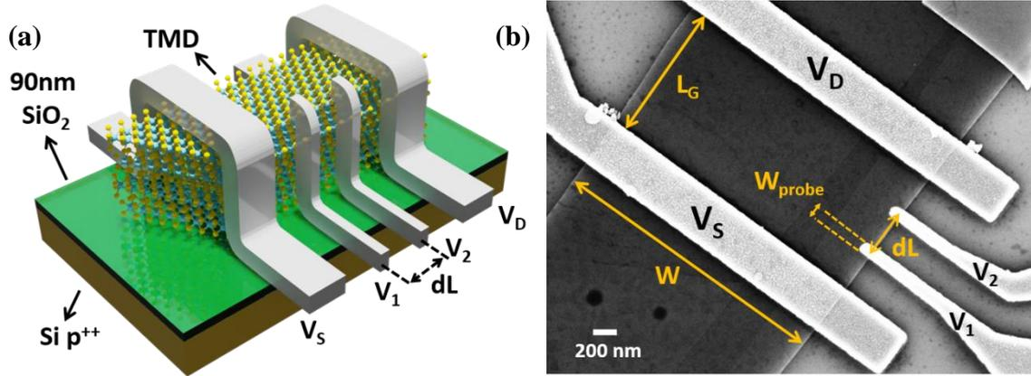
**Figure 1.** (a) A schematic illustration and (b) scanning electron microscope (SEM) image of a 4-terminal device structure, where  $L_G$  is the channel length,  $dL$  is the distance between two voltage probes  $V_1$  and  $V_2$ , and  $W_{\text{probe}}$  is the width of each voltage probe. When only  $V_S$  and  $V_D$  electrodes are used together with the gate electrode in the measurement, it is referred to as 2-terminal measurement.
