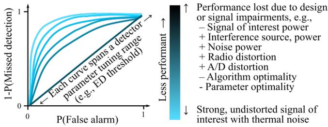
Fig. 3. ROC curves shown for a hypothetical sensor. Each represents the false alarm and missed detection tradeoff for a specific combination of sensing algorithm, hardware impairments, and radio environment.
