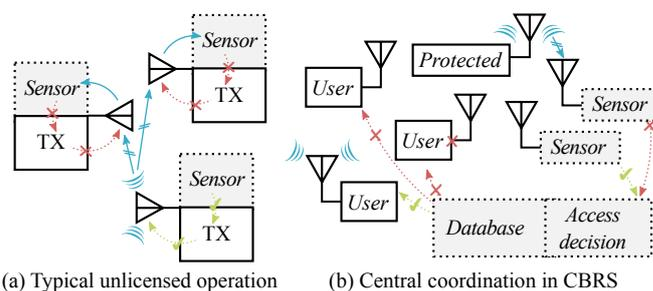
Fig. 2. Occupancy status based on incident radio transmissions (solid blue arrows) are detected by sensing nodes. These outputs (dotted lines) serve as feedback for dynamic spectrum access decisions in real-time. In unlicensed spectrum commons (a), each spectrum user is responsible for this sensing before transmission. Centrally-coordinated access in CBRS (b) depends instead on a distributed sensor network to protect incumbents.
