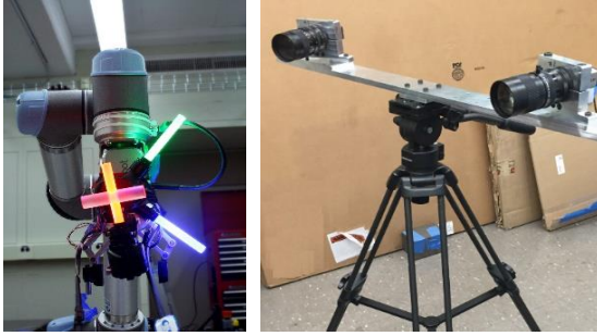
a) Smart target (mounted on the end effector of UR5) b) Vision-based measurement instrument
