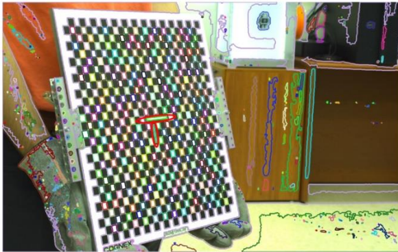
Figure 12. Detected contours from the stereo calibration image
