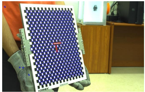
Figure 14. Improved detected corners from the stereo calibration image
