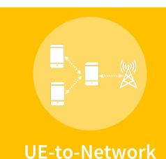
Allow devices to access the network using the D2D link with another device in proximity
