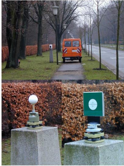
(b) Fig. 8 (a) Curtin University baseline in Western Australia. Reproduced from Lichti et al [25] with permission from Spatial Sciences Institute, Australia. b) Measurements made at the HAW baseline in Hamburg-Ohldorf, Germany – TLS shown on top (on pedestal next to the van) with sphere and special targets shown at the bottom. Reproduced from Kersten et al [73].
