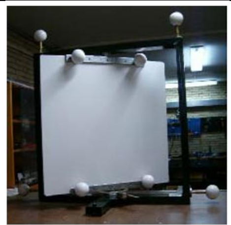
Fig. 25 Artifact to estimate effect of angle of incidence. Reproduced from Kersten et al [134].
