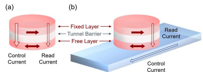
FIG. 1. Magnetic tunnel junctions (dark red arrows represent magnetization direction). (a) Standard magnetic tunnel junction with fixed and free layers and the control current following the same path as the read current. (b) magnetic tunnel junction grown on heavy metal layer with separate read and control current paths.
