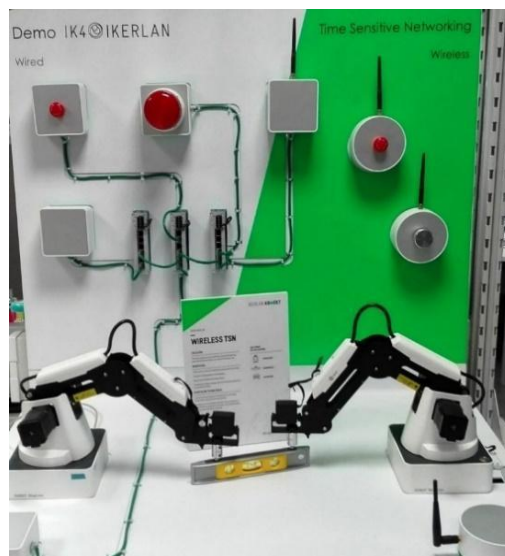
Figure 2. Wireless TSN applied to collaborative robotics
