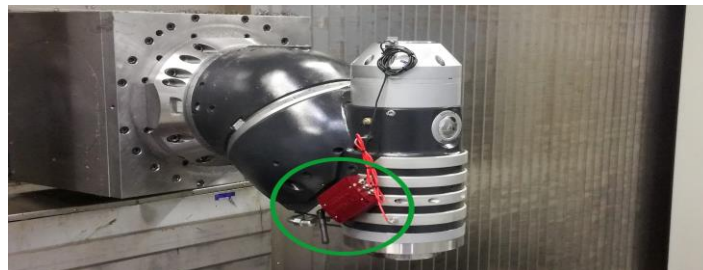
Figure 1. Milling machine monitored by a wireless sensor (used with permission by SORALUCE-IDEKO **).
