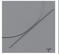
Figure 3. Silicon photonic crystal cavity thermometer fabricated at NIST
