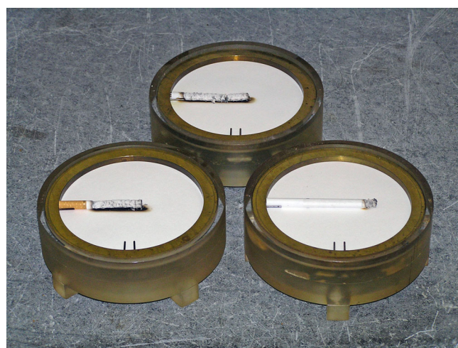
FIGURE 5 Photograph of typical results of determinations using ASTM E 2187-04 (NIST photograph). Top: full-length burn of a non-filter cigarette; Right: full-length burn of a filter cigarette; Left: ceased burning of a less fire-prone cigarette
