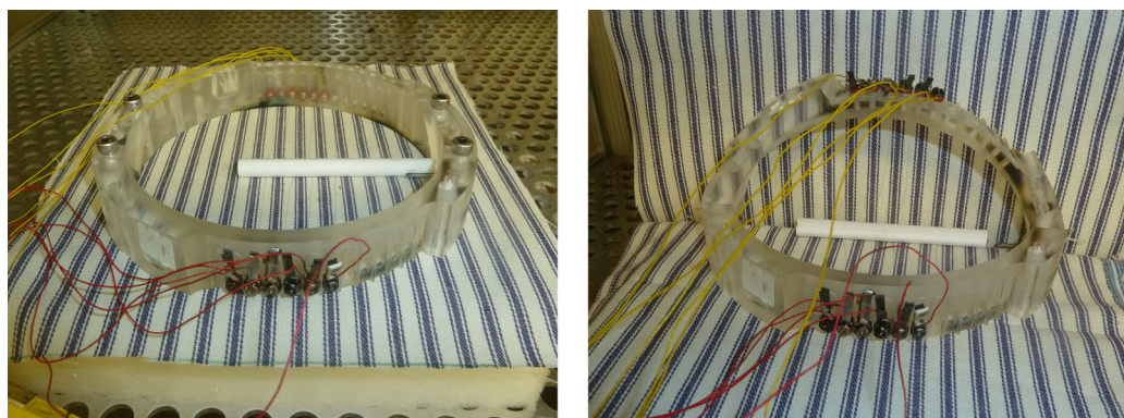
FIGURE 9 Photographs of flat (left) and crevice (right) substrates with fine thermocouples to characterize surface temperature distribution and spread rate
