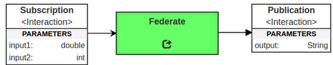
Fig. 2. An example WebGME Federate Model
