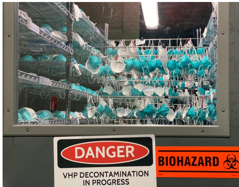
Figure 1: Battelle Memorial Institute VHP masks decontamination system. Photo used with permission (John Clay email 4/6/2020).
