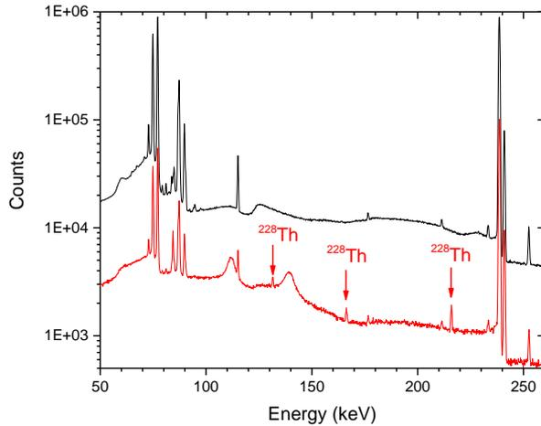
The resolution of HPGe allows identification of the weak  $\gamma$ -ray peaks from  $^{228}\text{Th}$  decay
