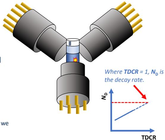
The  $^{224}\text{Ra}$  activity standard developed by NIST is based on TDCR counting. This is a self-calibrating, “primary”, liquid scintillation counting method. Measuring the number of triple- and double-coincidence events gives a measure of the counting efficiency. The source activity ( $A$ ) can then be calculated from the efficiency ( $\epsilon$ ) and count rate ( $N$ ):  $A = N/\epsilon$
