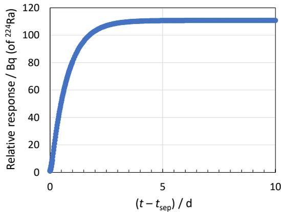
Ionization chamber response increases rapidly after separation as progeny grow in, meaning that any uncertainty on difference between  $t_{\text{sep}}$  and  $t_{\text{meas}}$  results in a very large uncertainty on the activity
