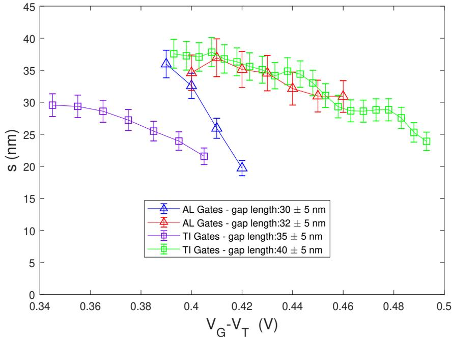
FIG. S3. Barrier widths,  $s$ , as determined from fitting to equation 3 of the main text and corresponding to the data presented in Figure 3 of main text.
