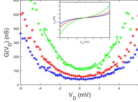
FIG. 2. 4-terminal DC transport data for a tunnel junction device. The inset shows the measured  $I(V_D)$  used to obtain the conductance ( $dI/dV_D$ ) through numerical differentiation that is plotted in the main panel. The blue, red, and green curves are taken at gate voltages of 0.87 V, 0.88 V, and 0.89 V, respectively. The lines are quadratic fits to equation 3 (see text). All data are taken at  $T = 2$  K.
