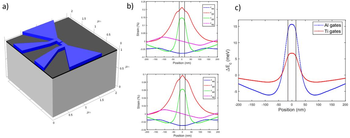
FIG. S1. (a) Schematic of the 3-dimensional device model used in COMSOL simulations for a device with a 25 nm thick gate oxide, 30 nm wide tunnel gap, and 100 nm wide gates. (b) Plot of various strain components Al (upper plot) and Ti (lower plot) gated devices at 2 K. (c) Plot of the conduction band modulation along the channel using the strain components in (b). The vertical black lines in (b) and (c) denote the edges of the gates.
