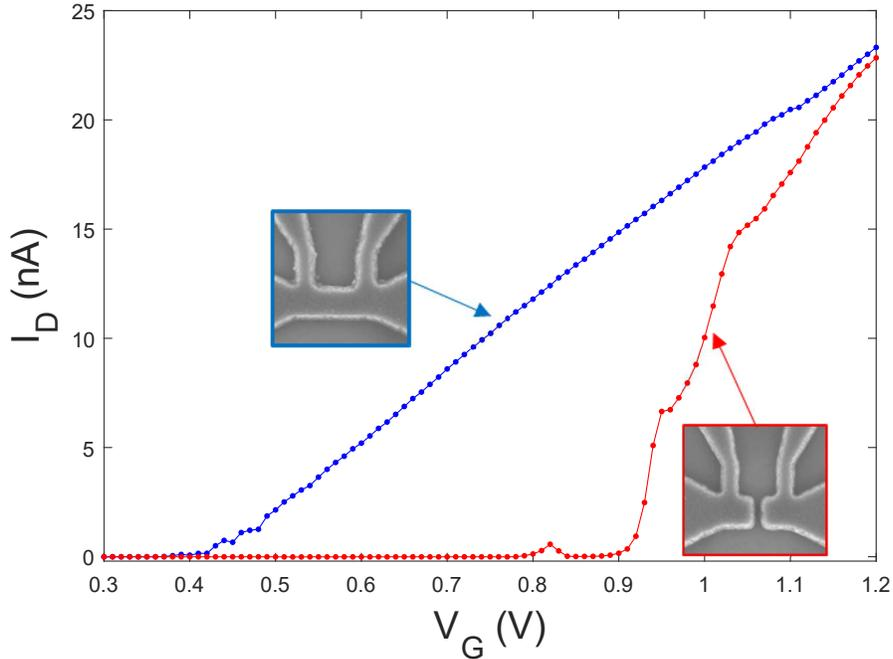
FIG. S2.  $I(V_G)$  for titanium-gated devices at 2 K and  $V_D = 1$  mV . The blue data is from a wire device with no gap in the gates and the red data is from tunnel junction device. The large gate voltage delay between the two devices is due the presence of the tunnel barrier.
