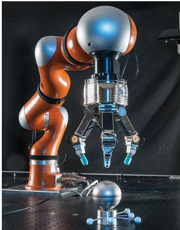
Figure 1: A collaborative robot attempting to grasp a metal sphere using a commercial 3D imaging system (top right).
