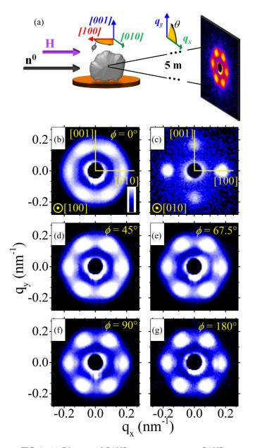
FIG. 1. (a) Diagram of SANS measurement setup. SANS patterns for (Fe, Co)Si initially aligned with the  $H \parallel [100]$  axis measured (b) with  $n^0 \parallel [100]$  and (c)  $n^0 \parallel [010]$ . SANS patterns with  $H \parallel n^0$  rotating the sample in the (001) plane by  $\phi = (d) 45^\circ$ , (e) 67.5°, (f) 90°, then (g) back to the initial orientation ( $\phi = 180^\circ$ ).
