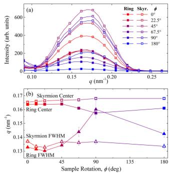
FIG. 3. (a) Summations of radial sector averages from Figs. 1(b) and 1(d)–1(g), taken at increments of  $60^{\circ}$  with  $\Delta\theta = \pm 3.5^{\circ}$  starting at  $0^{\circ}$  and  $30^{\circ}$ , capturing the radial distribution of the ring and skyrmion phases, respectively. Half of the data symbols are not shown for clarity. (b) Peak center and width for the sector averages of the ring and skyrmion features as a function of the sample rotation angle.
