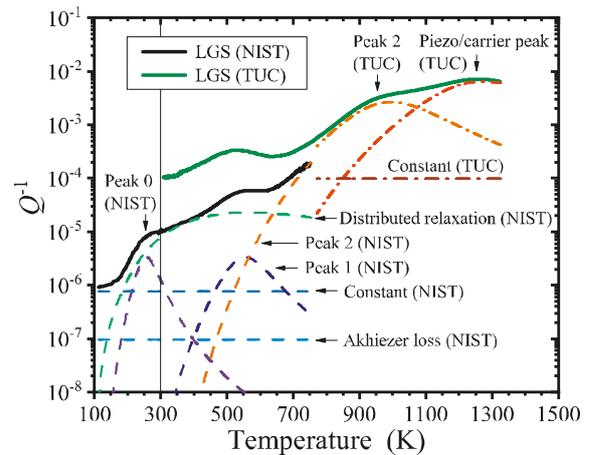
Fig. 1. Acoustic loss  $Q^{-1}$  of two LGS crystals measured at NIST and TUC. Resonant frequencies were 6.05 MHz (NIST) and 5.0 MHz (TUC) at ambient temperature. Dashed and dashed-dotted lines are contributions to  $Q^{-1}$  of the NIST and TUC crystals, respectively, determined from least-squares fits.
