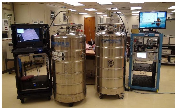
Fig. 1. Direct comparison between NIST transportable PJVS (left) and SCL PJVS (right)
