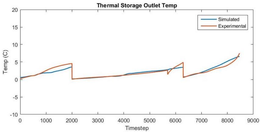
Figure 6: Thermal Storage Outlet Temperature for Discharging
