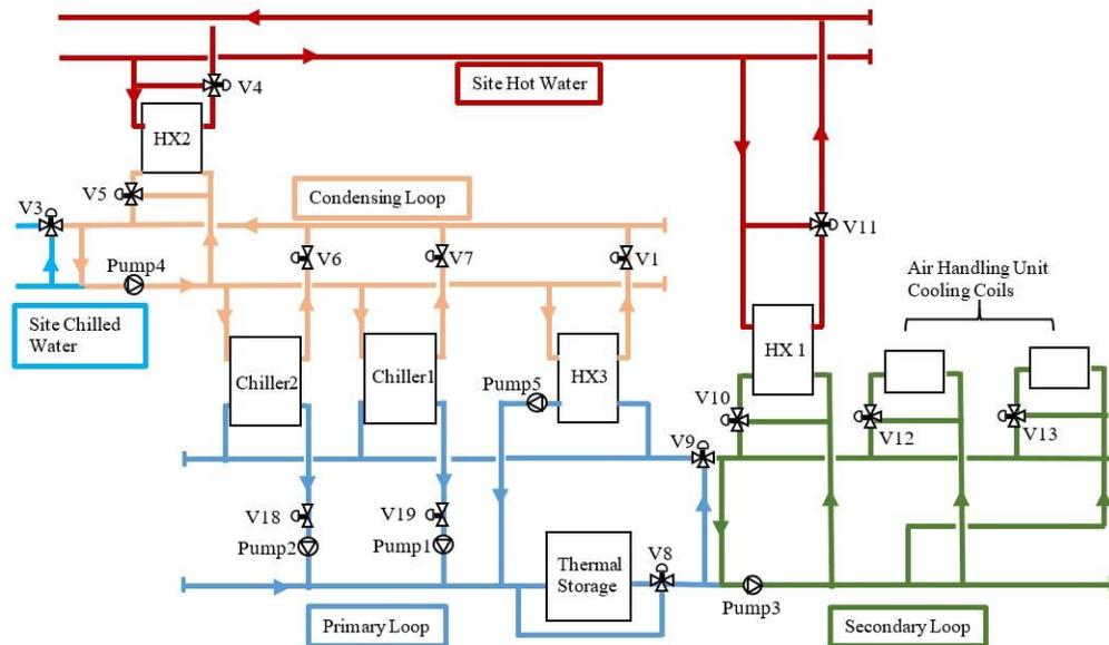
Figure 1: Schematic of the IBAL Hydronic System (Pertzborn 2015)
