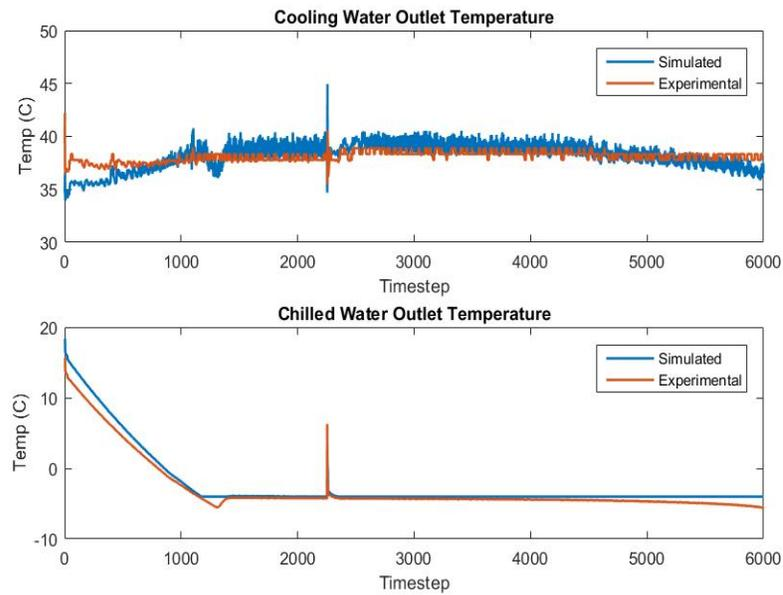
Figure 3: Chiller Outputs for Charging using Chiller 2
