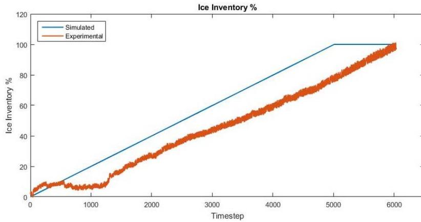
Figure 5: Ice Inventory Percentage for Charging using Chiller 2
