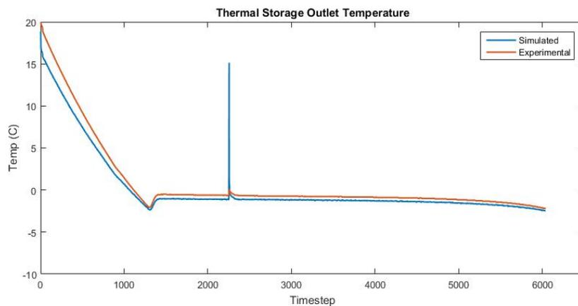
Figure 4: Thermal Storage Outlet Temperature for Charging using Chiller 2
