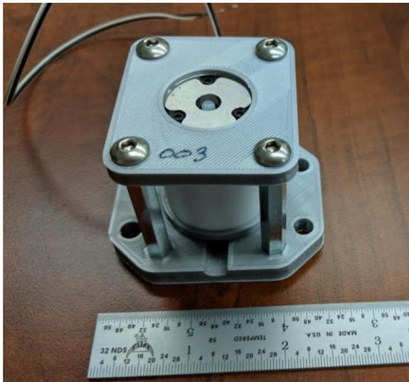
**FIGURE 2: POSITION VERIFICATION SENSOR WITH DISCRETE OUTPUT**
