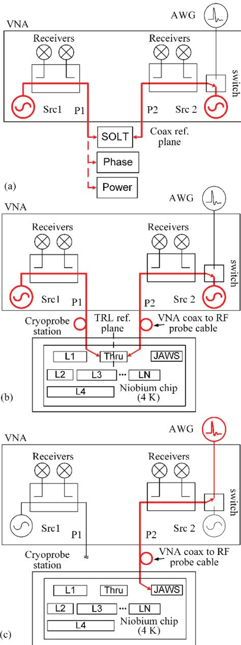
Fig. 2a) First-tier VNA calibration using SOLT, power and phase standards.
