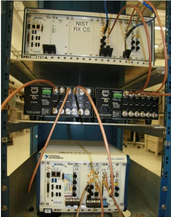
Fig. 3: Channel sounder hardware used for timing experiments. From top to bottom: receiver unit, pair of Rb clocks, and transmitter unit. In this image, the cables for PPS and 10 MHz timing signals are visible, but power, RF, and computer cabling are removed for clarity.
