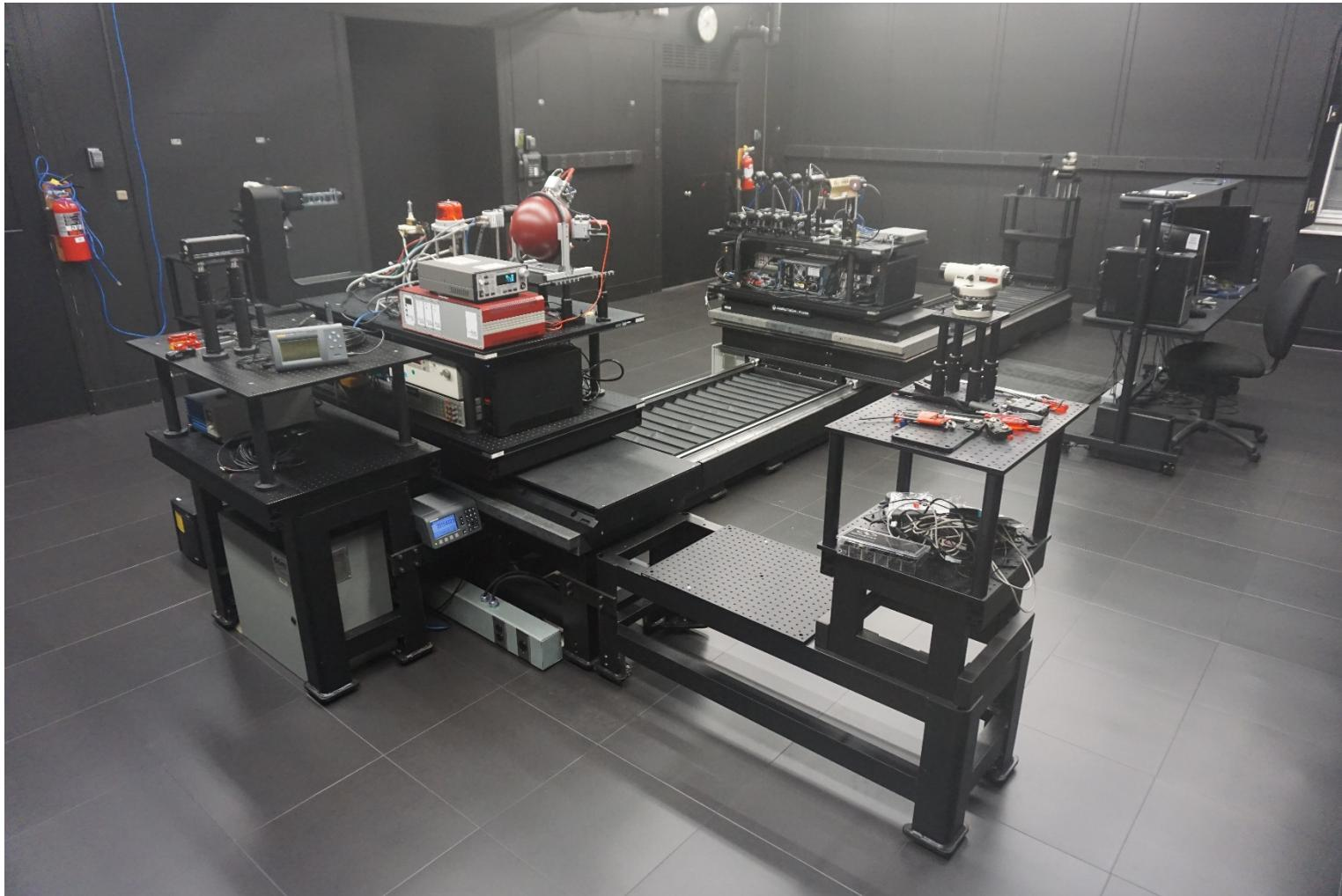
6 m ball screw, 5 m travel,  $\Delta d = 50 \times 10^{-6}$  m, with a source stage and sensor stage
