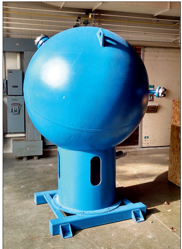
Fig. 1. The Big Blue Ball. It is made of carbon steel, has an inner volume of about 1800 liters, and weighs more than 1000 kg. (photo credit: NIST's Fluid Metrology Group).
