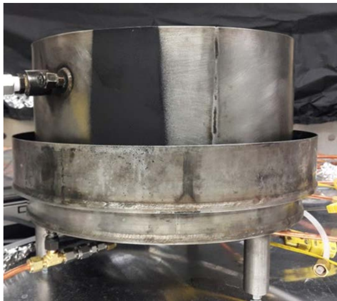
Figure 1. The 0.30 m diameter, water-cooled, stainless-steel, burner with fuel overflow section.
