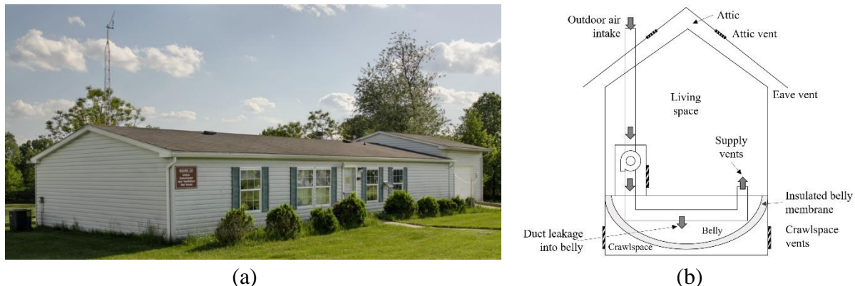
Figure 1. (a) Photograph and (b) schematic cross-section of MH showing crawlspace and belly.
