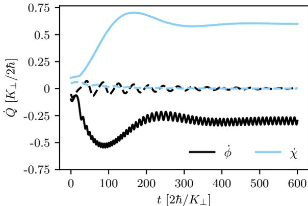
FIG. 3. Hysteretic dynamics of the DW as seen from two different stationary solutions of Eqs. (35),  $\dot{\phi}$  (black) and  $\dot{\chi}$  (blue/light gray) obtained numerically with the same system parameters  $\alpha = 0.5$ ,  $m = 50$  and  $j_t = 0.75$ . The two solutions have slightly different initial conditions, leading to a running state (solid lines) and damped state (dashed lines).
