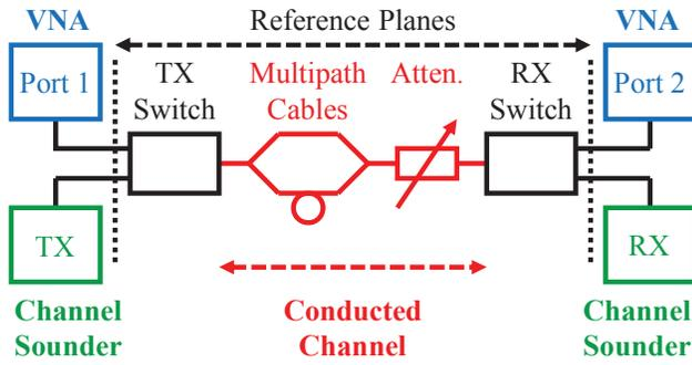
Fig. 1. Measurement setup.
