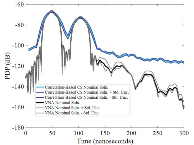
Fig. 2. Comparison of power delay profiles of the correlation-based channel sounder and VNA for multipath channel 1.
