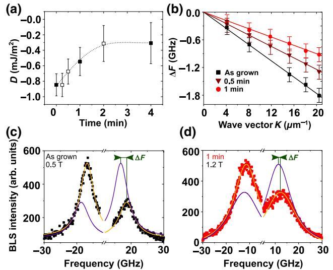
FIG. 3. (a) DMI constant  $D$  as a function of the biasing time; values calculated using estimated  $M_s$  values are shown as empty symbols. The dotted line is a guide to the eye. (b) Frequency asymmetry as a function of the wave vector, and linear fitting lines. BLS spectra at  $k = 20 \mu\text{m}^{-1}$  for the (c) as-grown and (d) 1-min-biased films. The solid lines correspond to a Lorenzian fitting.
