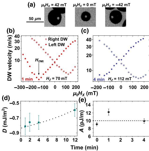
FIG. 4. (a) Kerr-microscopy images of domain expansion in the sample biased for 1 min under in-plane fields ( $\mu_0 H_X$ ). Velocity curves as a function of  $\mu_0 H_X$  from films biased for (b) 1 and (c) 4 min. (d) DMI parameter  $D$  extracted using the experimentally obtained values of  $A$  shown in (e). The lines are a guide to the eye.
