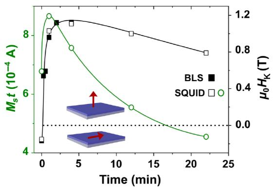
FIG. 2. (a)  $M_s \times t$  (circles) and (b)  $\mu_0 H_K$  (squares) as a function of the E-field biasing time. The lines are a guide to the eye.
