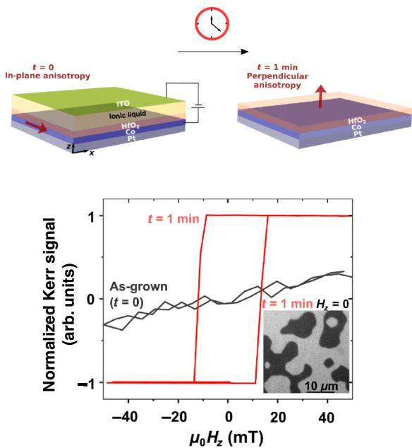
FIG. 1. Schematic of the Pt/Co/HfO<sub>2</sub> liquid gate device together with hysteresis loops measured in a perpendicular magnetic field before (black) and after (red) applying a gate voltage of  $-3$  V for 1 min. The Kerr-microscopy image (inset) shows the domain pattern in the demagnetized state after the gate voltage application.
