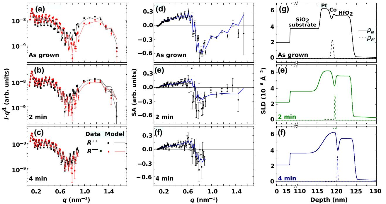
FIG. 7. (a)–(c) PNR signals  $R^{++}$  and  $R^{--}$  as a function of the wave vector, and the corresponding fitting lines; the spin asymmetry (SA) is plotted in (d)–(f). The scattering-length density (SLD), the model used to fit the experimental data, is presented in (g)–(i).
