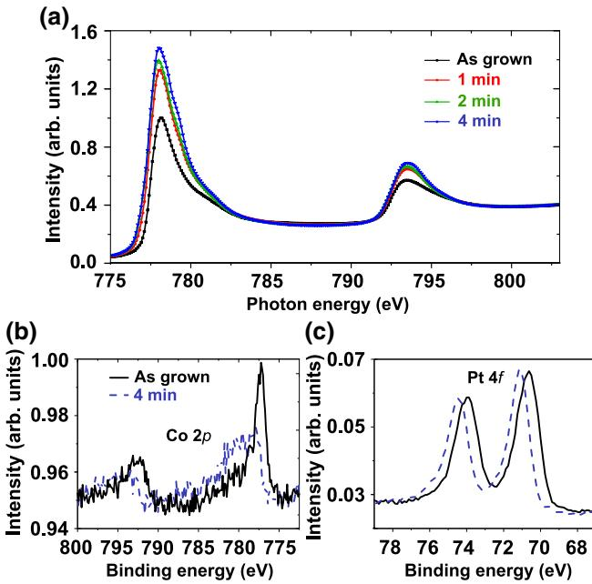
FIG. 6. (a) XAS spectra at the Co  $L_2$  and  $L_3$  edges as a function of biasing time. XPS spectra in the (b) Co  $2p_{3/2}$  and (c) Pt  $4f$  regions for an as-grown sample (solid lines) and a sample biased for 4 min (dotted lines).
