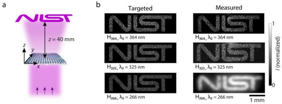
Figure 5: Spin-multiplexed near-UV self-accelerating beam generator.
