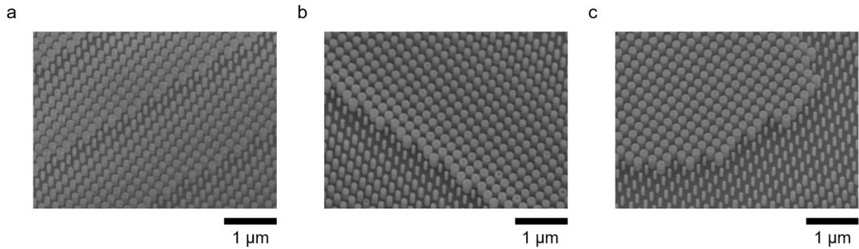
**Fig. S7.** Scanning electron micrographs (viewing angle:  $20^\circ$ ) of selected areas of polarization-independent metasurfaces designed for operation at  $\lambda_0 = 364$  nm. **a**, Metalens  $L_{364}$ . **b**, Self-accelerating beam generator  $B_{364}$ . **c**, Metahologram  $H_{364}$ .
