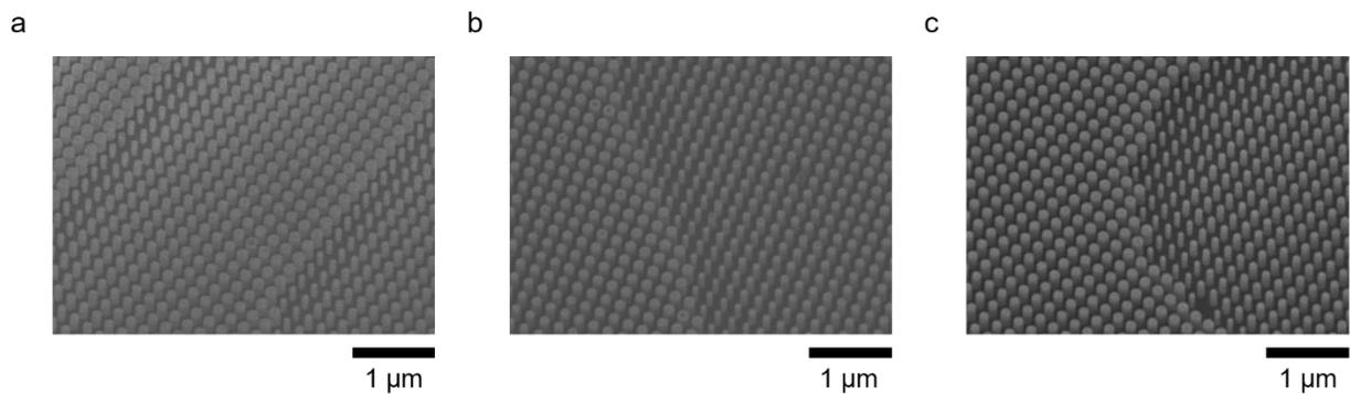
**Fig. S8.** Scanning electron micrographs (viewing angle:  $20^\circ$ ) of selected areas of polarization-independent metasurfaces designed for operation at  $\lambda_0 = 325$  nm. **a**, Metalens  $L_{325}$ . **b**, Self-accelerating beam generator  $B_{325}$ . **c**, Metahologram  $H_{325}$ .
