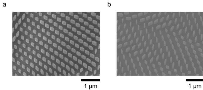
**Fig. S10.** Scanning electron micrograph (viewing angle:  $20^\circ$ ) of selected areas of spin-multiplexed metasurfaces designed for operation at  $\lambda_0 = 364$  nm. **a**, Metahologram  $H_{364}^{\text{spin}}$ . **b**, Self-accelerating beam generator  $B_{364}^{\text{spin}}$ .
