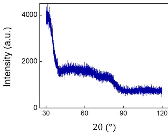
**Fig. S2.** X-ray diffraction (XRD) angular spectrum of ALD-deposited HfO<sub>2</sub>.
