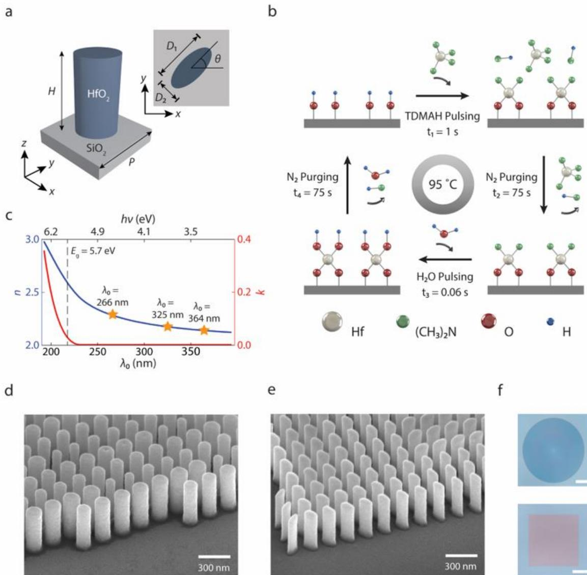
Figure 2: Polarization-independent near-UV metalenses.
