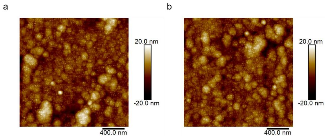
**Fig. S6.** Atomic force microscopy (AFM) characterization over the top surfaces of a patterned resist area (left) and non-patterned resist area (right) after the 200-nm-thick HfO<sub>2</sub> ALD coating. The scan is performed over a square area with side length of 2  $\mu$ m.
