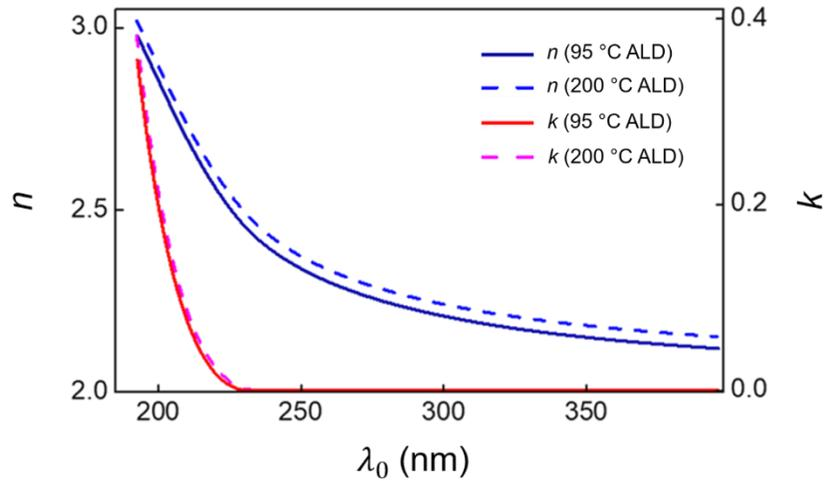
**Fig. S4.** Measured refractive index  $n$  and extinction coefficient  $k$  of HfO<sub>2</sub> films deposited by ALD at 95 °C and 200 °C, respectively.
