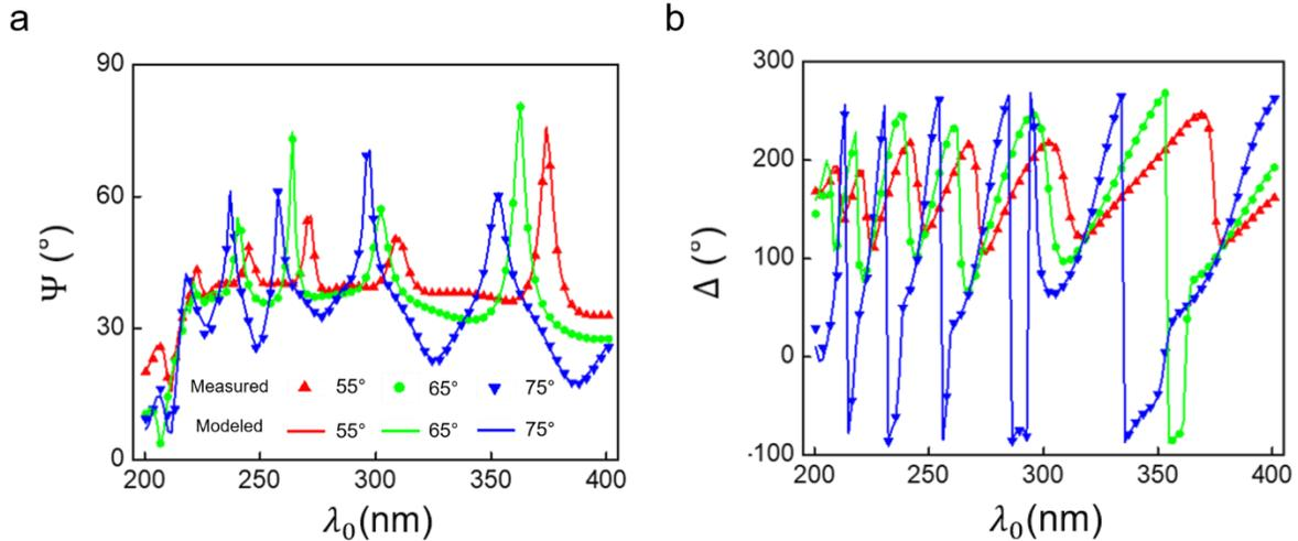
**Fig. S3.** Measured and best-match modeled Psi and Delta curves for ellipsometric characterization of low-temperature ALD-deposited HfO<sub>2</sub>. The legend in Fig. S3a applies to Fig. S3b.
