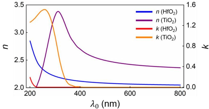
**Fig. S5.** Measured refractive index  $n$  and extinction coefficient  $k$  of the 95°C-ALD-deposited HfO<sub>2</sub> films and the 90°C-ALD-deposited TiO<sub>2</sub> films in the UV and visible range.
