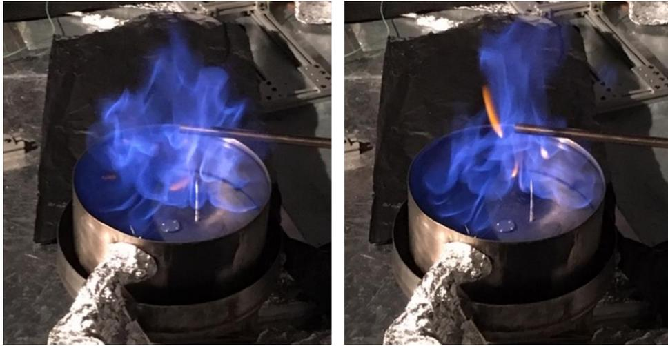
**Figure 4.** Images of pulsing methanol pool fire (30 cm diameter)
