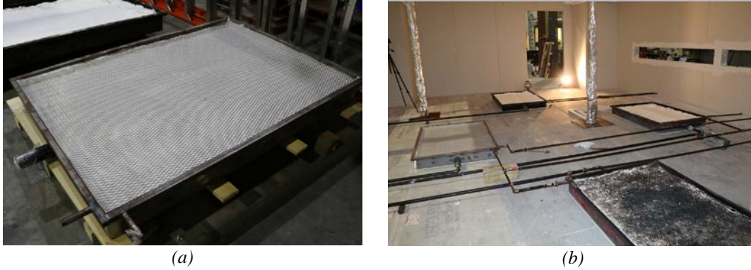
Figure 11. (a) The burner and (b) the position of the burners in the compartment.
