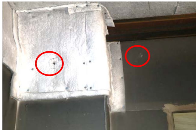
Figure 15. The heat flux gauges mounted in the south-east of the compartment.
