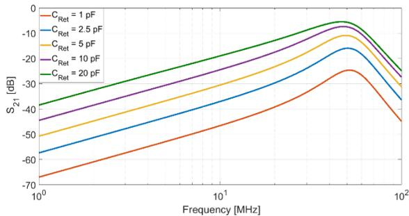
Figure 4. Forward transmission coefficient for various  $C_{Ret}$
