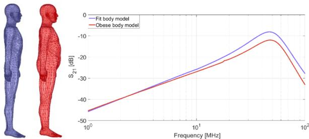
Figure 8. Forward transmission coefficient for various body shapes
