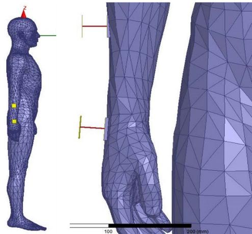
Figure 1. HBC electrodes on the right arm
