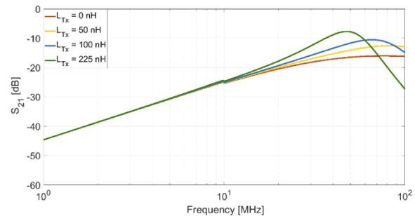
Figure 5. Forward transmission coefficient for various parasitic inductance
