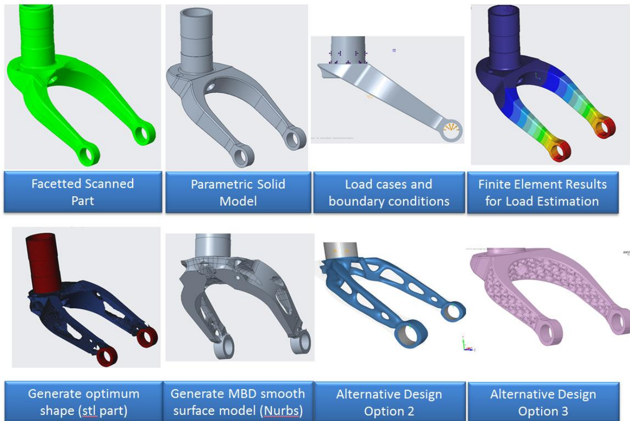
Figure 1 Technique that reduces weight and improves safety margins and reintroduces part's TDP into the Digital Thread.
