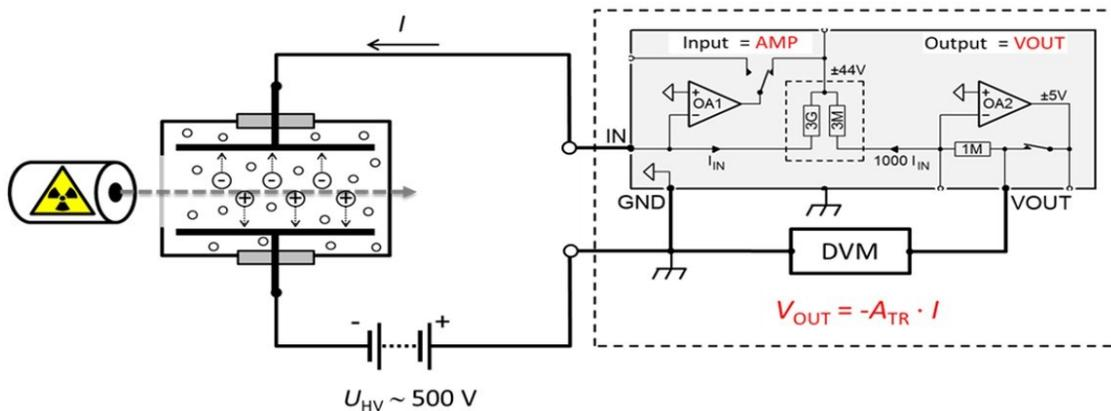
**Figure 4** Example operation of a ULCA in an electrometer mode for current measurements on an IC (left), with  $A_{TR} = 1 \text{ G}\Omega$  (using the internal  $1 \text{ M}\Omega$  resistor for current-voltage conversion) and for currents up to  $\pm 5 \text{ nA}$ . Note, the IC shown uses an external source, but the principle is the same for re-entrant ICs.
