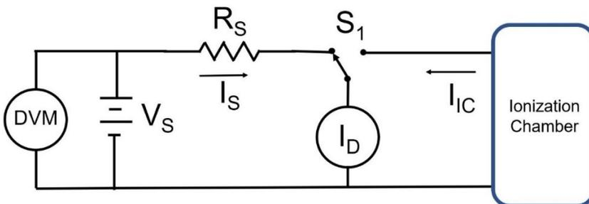
**Figure 5** Circuit diagram for calibration of an electrometer used with an ionization chamber. Switch S1 connects the electrometer to the ionization chamber or the voltage source, DVM, and standard resistor. See text for definition of other symbols. A calibrate, measure, calibrate sequence is used to bracket ion chamber measurements with before and after calibrations of the electrometer.
