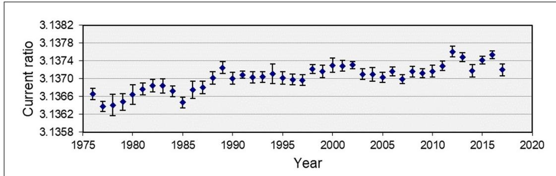
Figure 2) while the measured current produced by a single reference source has been stable only to 0.1 %. However, a long-term trend in the ratio can be observed— origin of this effect is unknown. Exacerbating the problem, it is likely that many laboratories will no longer be able to keep usual electrometers or reference sources for as long as 40 years (“forever”), making it even more important to have highly stable IC current measurement systems linked to the SI.
