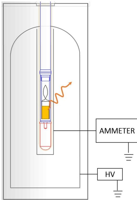
**Figure 1** Schematic diagram of an ionization chamber, showing a radioactive solution (yellow shaded), which emits a  $\gamma$ -ray (orange arrow) that is absorbed in the pressurized gas region. The resulting current is measured with the ammeter.
