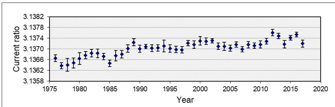
**Figure 2** Ratio of the current produced by two  $^{226}\text{Ra}$  sources as a function of time since 1976 at the BIPM, showing that a reproducibility of the order of 0.1 % can be achieved. However, a long-term trend in the ratio can be observed- the origin of this effect is unknown.
