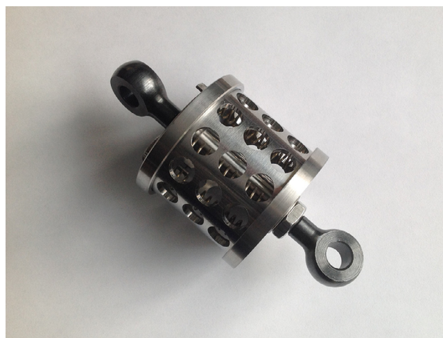
Fig. 3. Diving unit used for SBSE 2 procedure.
