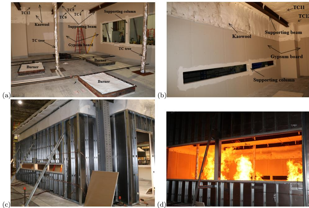
**Fig. 13** Photographs of the test compartment. Note that the door in (c) is for construction and transportation purpose and is closed during the test.
