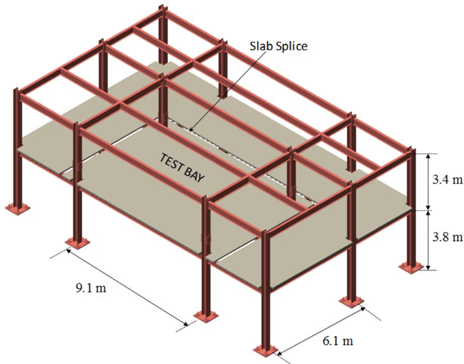
**Fig. 1** Proposed test frame for the NFRL composite floor project. The compartment studied in this paper is located in the test bay.
