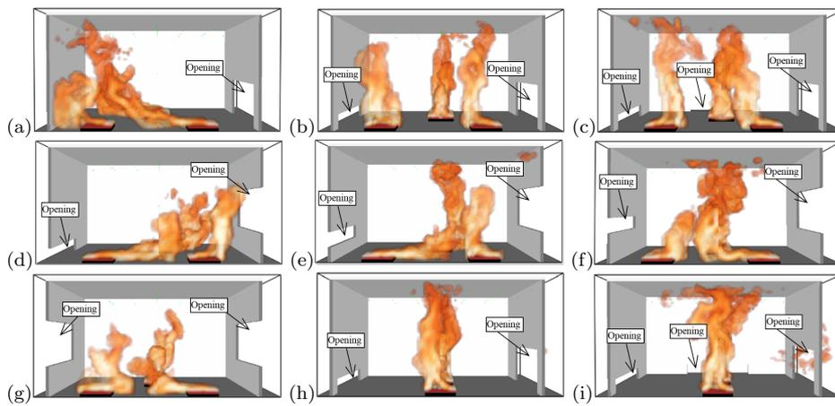
**Fig. 7** Field fire model simulated flame behaviors for various opening and burners configurations. Using symmetry, only half of the compartment is modeled and the “MIRROR” boundary condition is used in the symmetry plane [49]. Uniform grids of 0.1 m are used in the XYZ directions.
