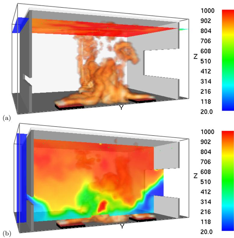
**Fig. 9** Field fire model simulated temperature distributions for the compartment with proposed HRR, opening, and burners (Units in °C). The results are for fire at 1 h after burning. (a) 30.5 cm below the ceiling; (b) 2 m away from window center.
