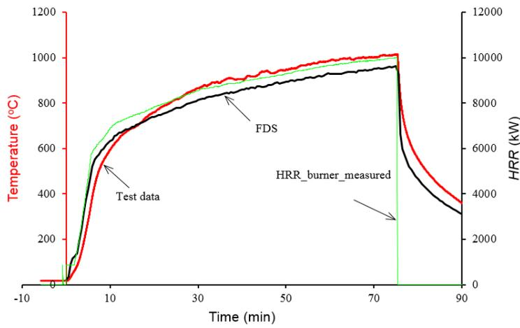
**Fig. 16** Comparison between the measured average gas temperature curve vs the FDS predicted curve using the measured heat release rate (of the burner). The zero of the X-axis is shifted 5.75 min from the ignition time.
