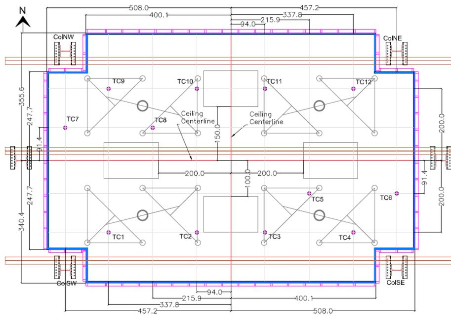
**Fig. 3** Plan view of the fire compartment. TC1 to TC12 are stainless-steel sheathed thermocouples placed 30.5 cm below the ceiling (Units in cm). Four rectangular boxes are the seats for natural gas burners. Triangles show the mechanical loading systems (not included in the fire tests reported in this paper).
