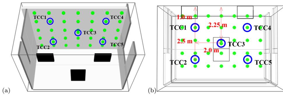
**Fig. 12** Thermocouple devices used to calculate the average gas temperatures by FDS. All the devices are located 30.5 cm below the ceiling. The circled five devices (TCC1 to TCC5) are used in the calculation. Comparison study shows that the average of these five devices is close to that of the 35 devices located 30.5 cm below the ceiling as shown (the green points).
