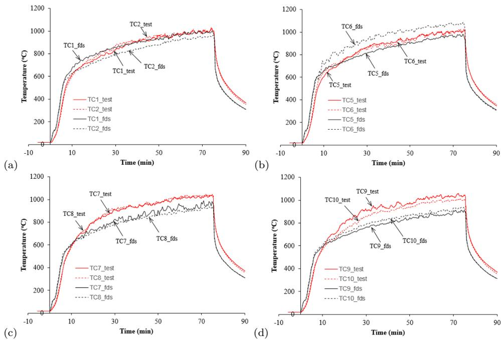
**Fig. 17** Comparison between measured and predicted gas temperatures by thermocouples located 30.5 cm beneath the ceiling. The zero of the X-axis is shifted 5.75 min from the ignition time. Data for TC3, TC4, TC11 and TC12 are not show for symmetry reason.
