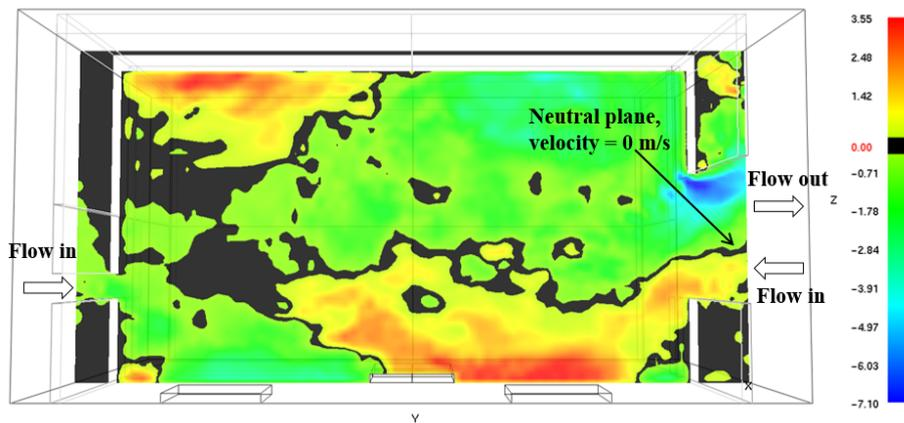
**Fig. 8** Field fire model simulated velocity distribution for the compartment with a main opening on the south wall (see Figure 1) and a small opening on the opposite north wall (Units in m/s, for black areas, velocity = 0 m/s). The objects only show outlines. The vertical slice is located at 2.0 m ( $X=2.0$  m) away from the symmetry plane.
