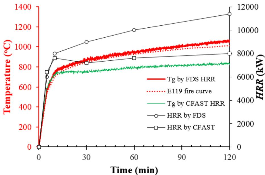
**Fig. 11** FDS predicted average gas temperatures and the *HRR* curves calculated by CFAST and FDS. The standard deviation among 35 temperature detectors located 30.5 cm below the ceiling is within 50 °C.
