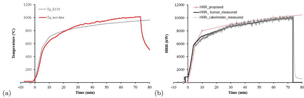
Fig. 15 (a) Comparison between measured average gas temperature curve vs the E119 fire curve; (b) Comparison between measured and proposed  $HRR$ . “calorimeter” – measured by cone calorimeter; “burner” – calculated based on natural gas flow velocity.
