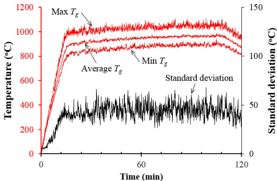
**Fig. 10** Field fire model predicted gas temperatures for the compartment with proposed *HRR*, opening, and burners. Max, Ave and Min  $T_g$  are maximum, average, and minimum values of 35 thermocouples located 30.5 cm below the ceiling.
