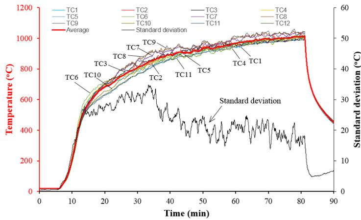
Fig. 14 Test data for twelve thermocouples.
