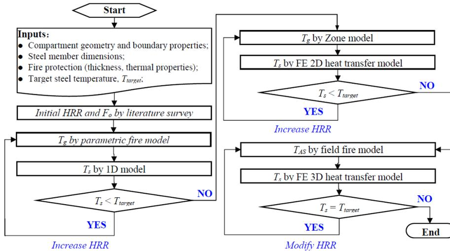
**Fig. 2** Procedure for determining a heat release rate and vent configuration to reach a target temperature in a steel member exposed to fire.  $T_{target}$ ,  $T_g$ ,  $T_s$  and  $T_{AS}$  are target temperature, gas temperature, steel temperature and adiabatic surface temperature, respectively.  $HRR$  could vary or not vary with time, depending on the user's assumption.
