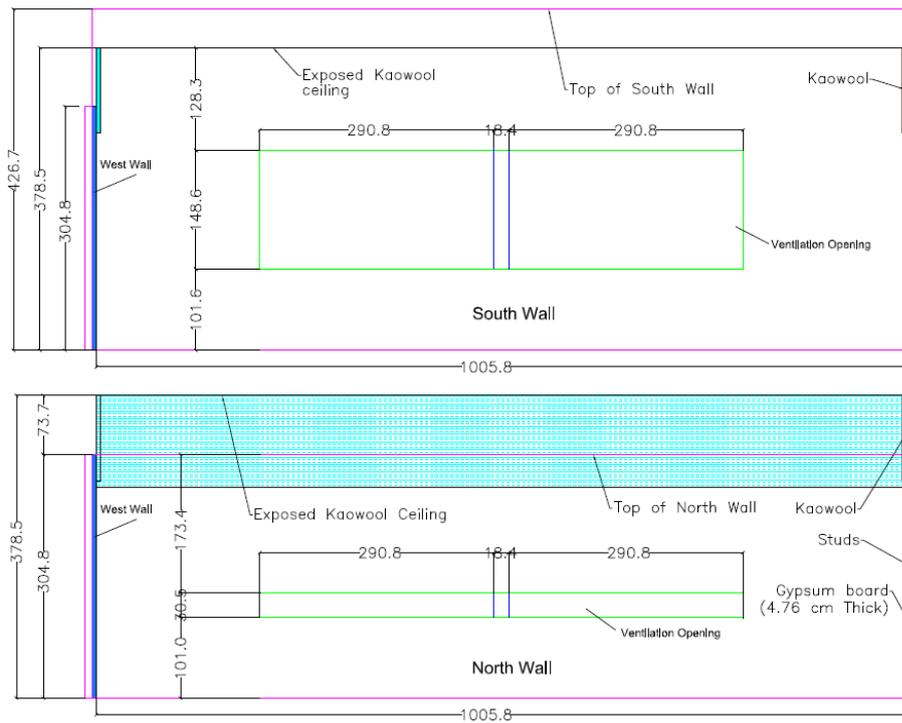
**Fig. 4** Elevation view of the fire compartment (Units in cm). The compartment walls are made of stiffened sheet steel (18 gauge) protected by three layers of 16 mm thick gypsum boards and the compartment ceiling slab are made of stiffened sheet steel (20 gauge) protected by two layers of 25.4 mm thick ceramic blanket (kaowool). Two layers of 16 mm cement boards are placed on the floor of the compartment for insulation purpose.
