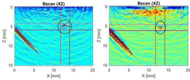
Figure 6. PAUT/FMC/TFM images of the cylinders with different orientations ( $\varnothing$  0.30 mm, L 2 mm) of the SS full-size star artefact, S1 design
