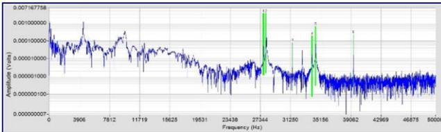
Figure 4. RAM typical spectrum of a SS half-size star artefact (the green vertical lines display the selected criteria)
