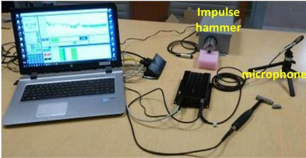
Figure 3. RAM set-up
