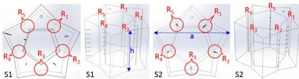
**Figure 1. Schematics of the AM star artefacts (design S1 and S2) proposed by the JG59 (where R is a Region in the artefact, “h” and “a” define the height and width of the artefact, respectively)**
