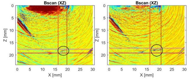
Figure 10. PAUT/FMC/TFM images of the horizontal cylinders, of 700  $\mu$ m (left) and 400  $\mu$ m (right), open to outside and located on the outer side of the SS full-size star artefact, S2 design
