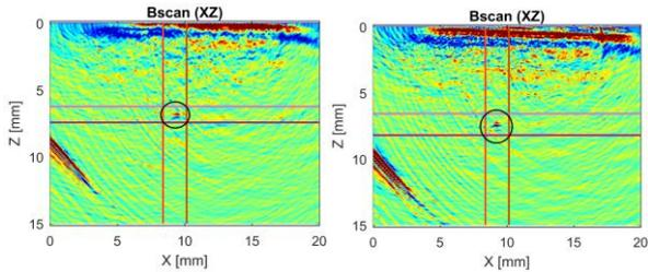
Figure 8. PAUT/FMC/TFM images of the spheres of 700  $\mu$ m (left) and 400  $\mu$ m (right) of the SS full-size star artefact, S1 design
