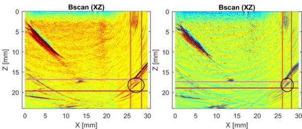
Figure 9. PAUT/FMC/TFM images of the horizontal cylinders, of 700  $\mu$ m (left) and 500  $\mu$ m (right), open to outside and located on the inner side of the SS full-size star artefact, S2 design
