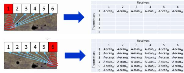
Figure 5. Principle of data acquisition with FMC
