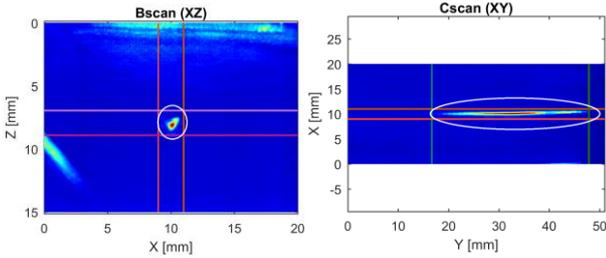
Figure 7. PAUT/FMC/TFM images of the vertical cylinders from the top (left) and from the side (right) of the SS full-size star artefact, S1 design
