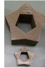
**Figure 2. Stainless steel star artefacts, full-size: h=45 mm and a=60 mm, half-size: h=22.5 mm and a=30 mm**
