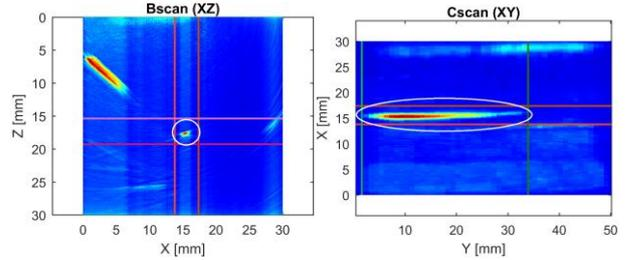
Figure 11. PAUT/FMC/TFM images of the vertical cylinders from the top (left) and from the side (right) of the SS full-size star artefact, S2 design
