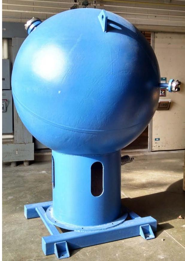
**Figure 1.** The 1.85 m<sup>3</sup> BBB is welded to and supported by a cylindrical pedestal. Two flanged ports are visible. The BBB's wall is 19 mm (3/4 inch) thick; the pedestal is made from 6.3 mm (1/4 inch) thick plate.
