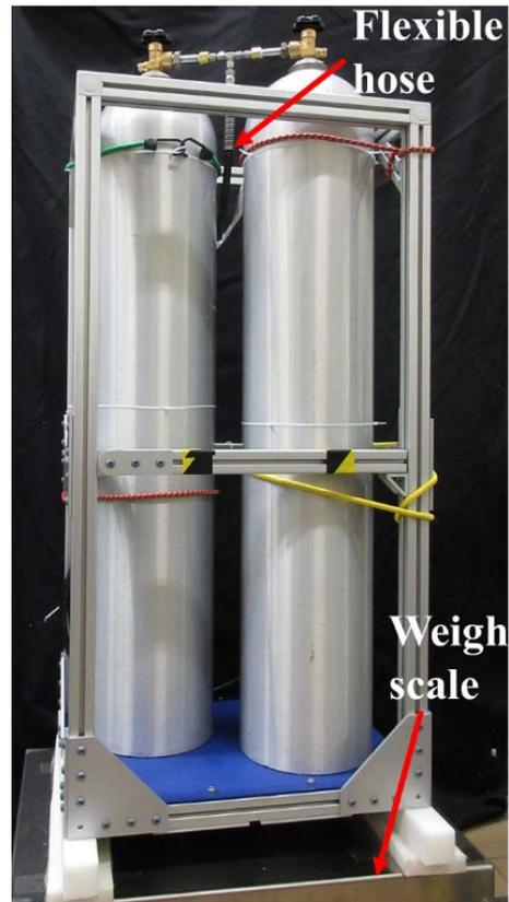
**Figure 3.** Weighing apparatus used to validate mass measurements using acoustic resonance frequencies.
