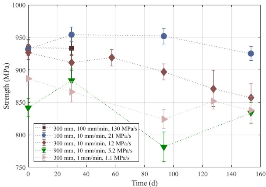
Figure 1. Weibull ultimate strength scale parameters, with the 95% maximum likelihood estimated confidence interval plotted as error bars. Specimens are all 30 mm wide, with varying gauge lengths and loading rates, as specified. Each group consists of at least 30 specimens.
