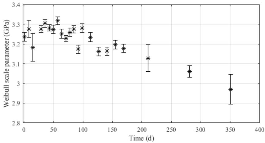
Figure 2. Weibull ultimate strength scale parameters, with the 95% confidence interval plotted as error bars, of aramid yarns after ageing at 70 °C and 76 % RH. The gauge length was 79 mm and the crosshead testing speed was 23 mm/min. Data is from [16]. Datapoints with small error bars consist of 50 specimens each, while datapoints with larger error bars consist of 15 specimens each.
