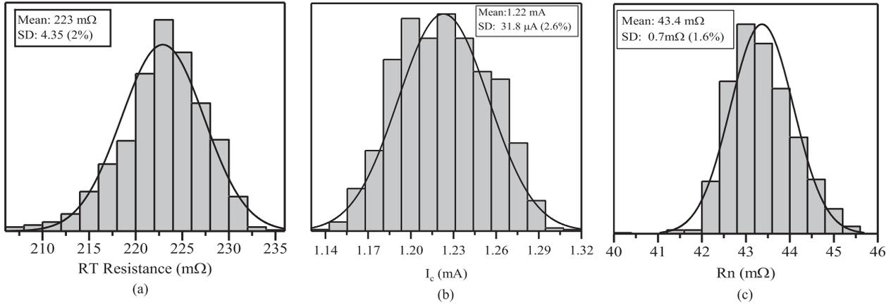
Fig. 2. Statistical distribution of the 1024 JJs measured. (a) RT resistance measurements with a mean resistance of 223 mΩ and a standard deviation of 2%. (b) Distribution of  $I_c$  with a mean of 1.22 mA and standard deviation of 31.8 μA. (c) Normal resistance measured at 4 K with a mean value of 43.4 mΩ and standard deviation of 1.6%. The solid curve is a fit of a normal distribution.
