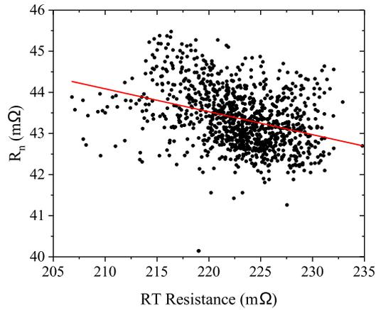
Fig. 6. Plot of the 4 K normal resistance versus RT resistance. There is a little correlation between  $R_n$  and the RT resistance. This lack of correlation is caused by random variations in process sizes resulting in different spreading resistance contributions for individual devices.
