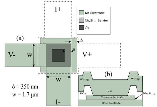
Fig. 1. (a) Layout of a CBKR studied in this paper. The top electrode is drawn wider for clarity. In the actual fabricated devices both electrodes had the same nominal dimensions. (b) Cross-section of a device in this paper. The via + counter electrode thickness was 450 nm.
