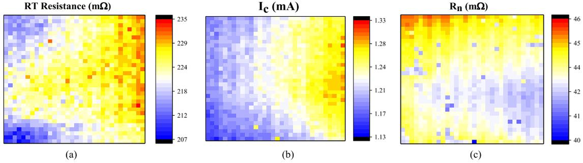
Fig. 4. Spatial distributions over a  $1 \times 1$  cm die of (a) RT resistance, (b) critical current  $I_c$ , and (c) normal resistance,  $R_n$ , at 4 K. Each square is an individual JJ in the  $32 \times 32$  array.
