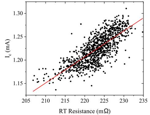
Fig. 5. Plot of  $I_c$  versus RT resistance.  $I_c$  exhibits a weak correlation with the RT resistance, which is the opposite behavior expected. Red line is a linear fit for the data.
